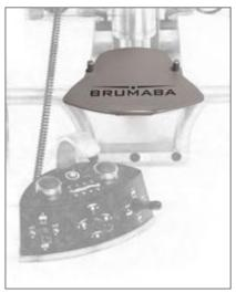
I For positioning the foot control on the undercarriage 4-EASY-DRIVE, 5-WHEEL-DRIVE
