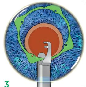
**4** Capture the hinge between the prongs of the Insertor.
