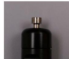
NOTE: Before reattaching the transducer, be sure that the connector interior for both the probe and transducer are completely dry (i.e. after cleaning). Also, ensure that the connector interiors are completely dry before storage.
